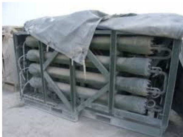
Figure 9: Military ROWPU (Reverse Osmosis Water Purification Unit)
